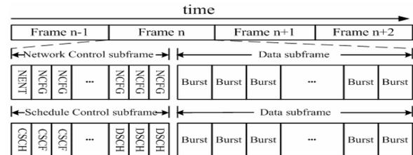
Fig. 1: Frame structure in Mesh mode
